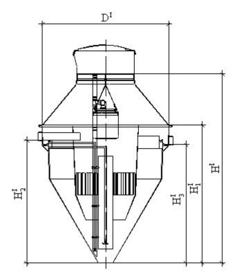
Figure 2. The main overhaul dimensions of the NV 1÷4m type treatment plant
