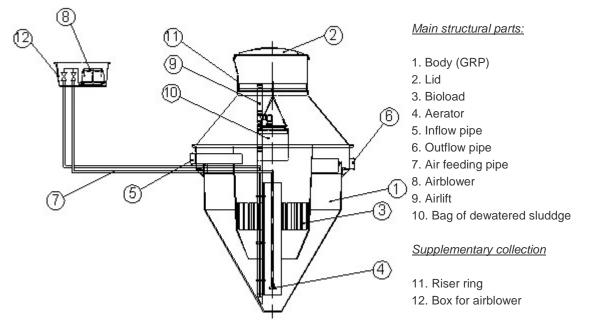
Figure 1. NV 1:4m type biological treatment plant with bags of dewatered sludge
